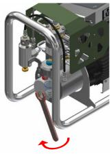
3. Replace crank oil cap. **Ensure to not over tighten** as this could damage the seal
