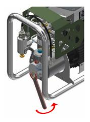
2. Undo crank oil cap with 27mm spanner and allow oil to flow out into container
