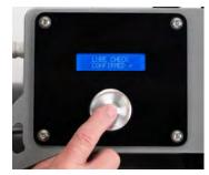
The display will then change to "set pressure". A default pressure of 100BAR (1450PSI/10MPa) is displayed.
